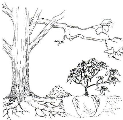
Figure 2: Root severance as a result of planting within RPA
