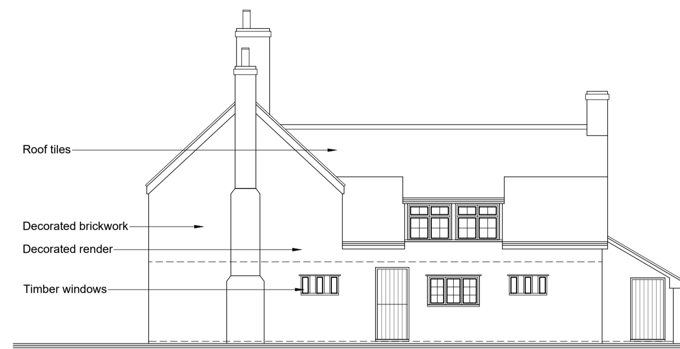
Side Elevation North East
