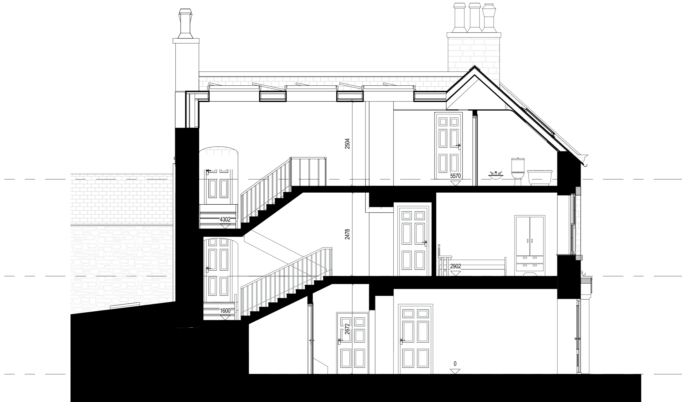
Figure 61. Existing Longitudinal Section
