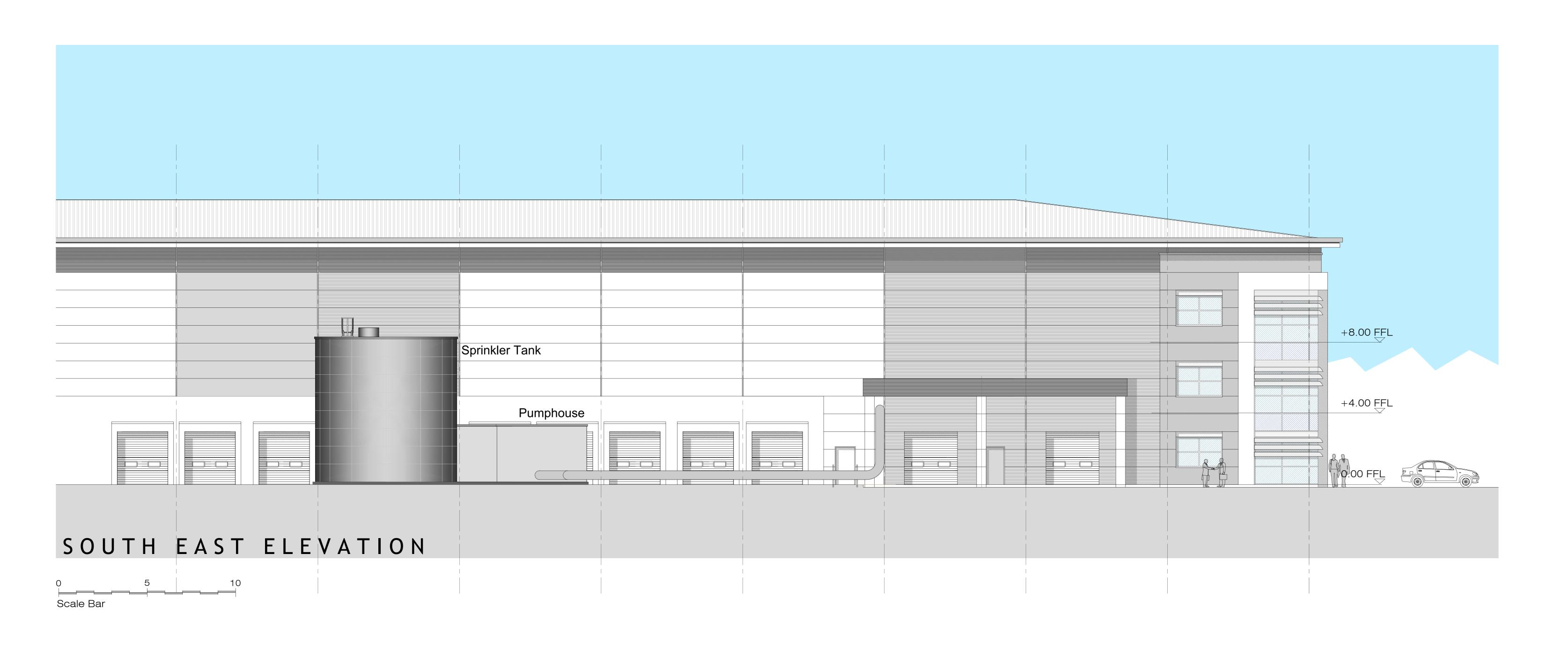
Proposed Materials Sprinkler Tanks and Overground Pipes: Galvanised metal.
