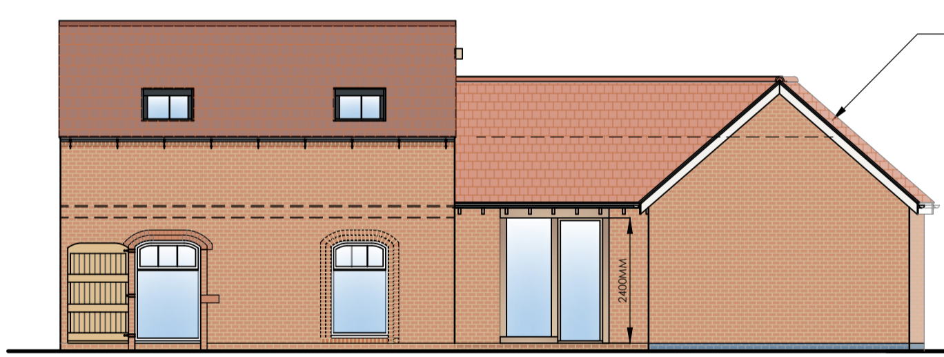
PROPOSED REAR ELEVATION OLDE BARN : 1/100
