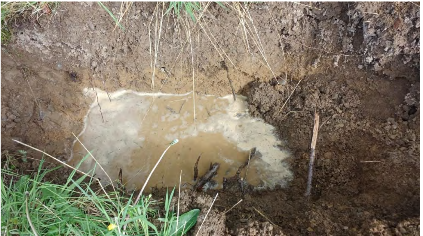
Photo 2 – Test hole 1 – 600mm deep. 300mm water level.
