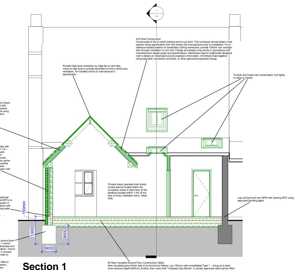
Unless otherwise noted provide: 1 layer of Celotex FR5000 (100mm) insulation board fixed between rafters and multi foil quilt to underside of rafters, fixed and held with 50x25mm counter batten fixed thorough into rafters above. Fix 12.5mm foil backed plasterboard ceiling and skim to the battens. Maintain airway gap into roof void using proprietary Glidevale Products or similar approved in conjunction with ventilators.
