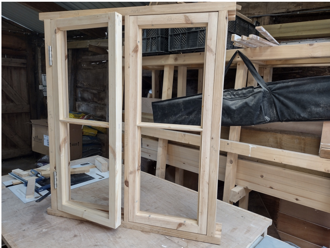
Exterior view showing flush casement finish to match existing
