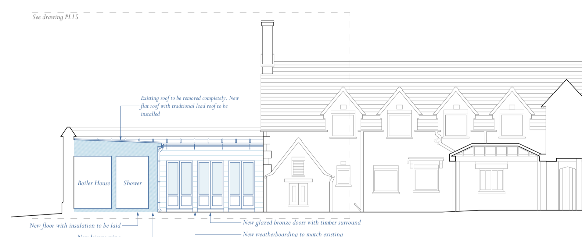
COURTYARD ELEVATION 4 (WEST)
