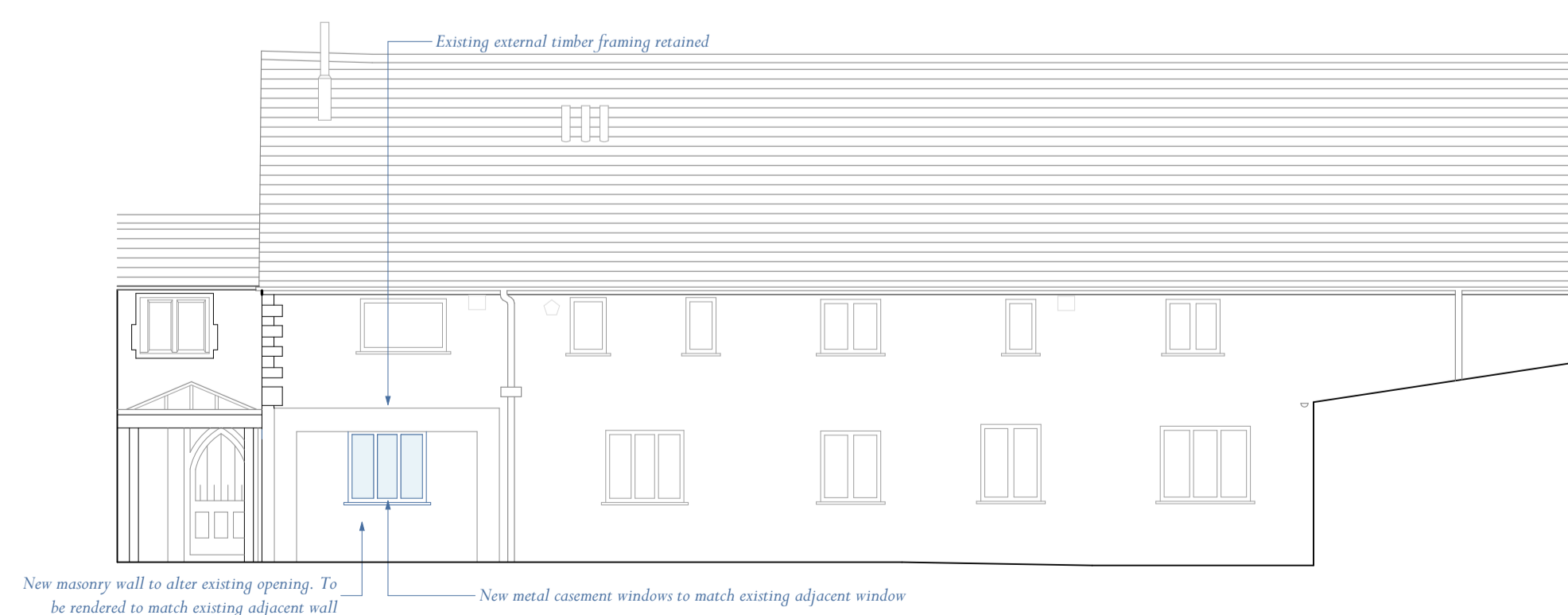
COURTYARD ELEVATION 3 (NORTH)
