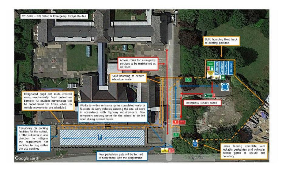
All roads and footpaths will be constantly monitored throughout the works. They will be cleaned, as necessary, with further wheel wash controls situated and used at both vehicles' entrances to ensure that any build-up of harmful materials does not present a hazard by being tracked onto the local highways.
