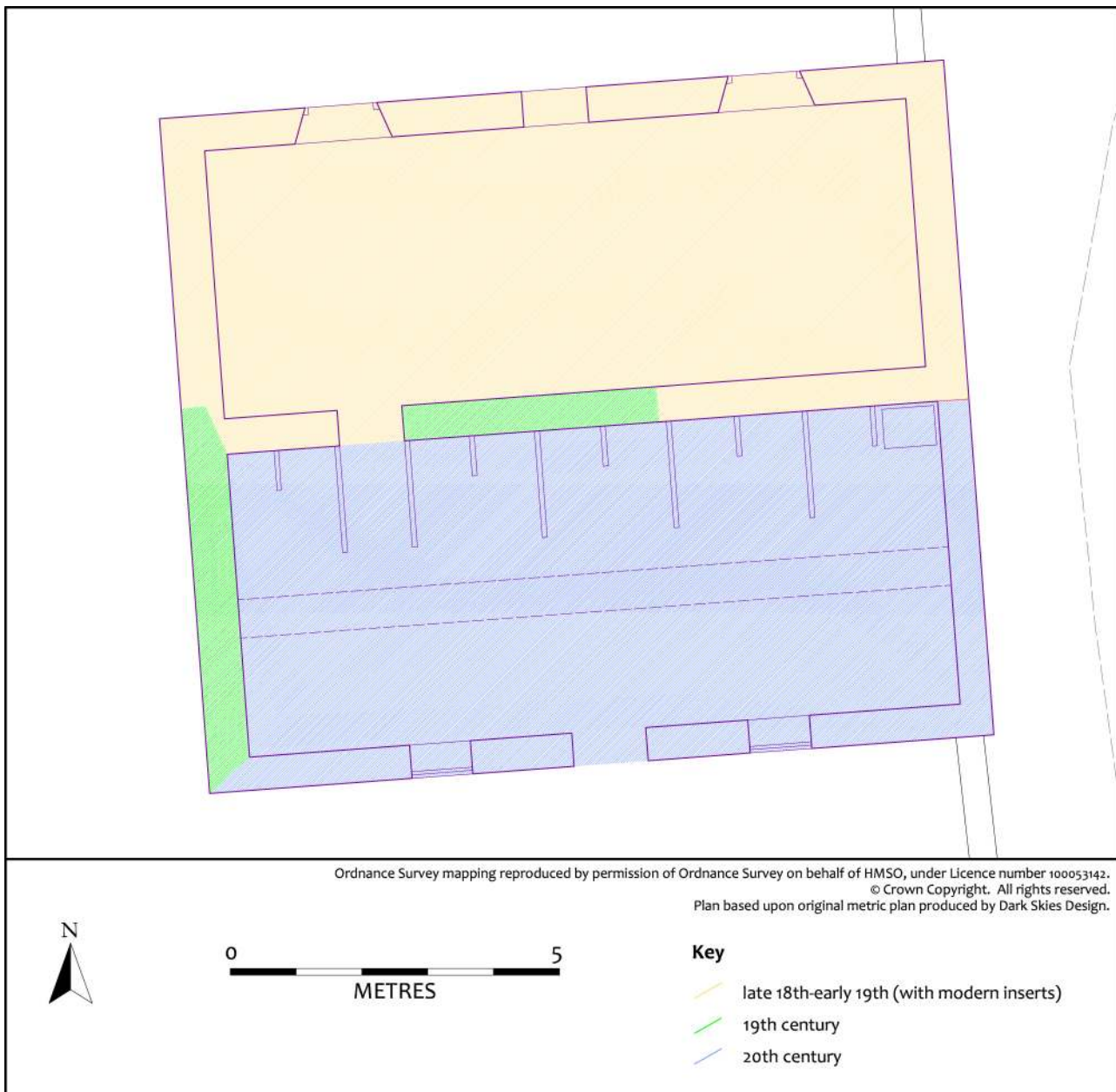
Figure 12. Suggested phasing of the present structure
