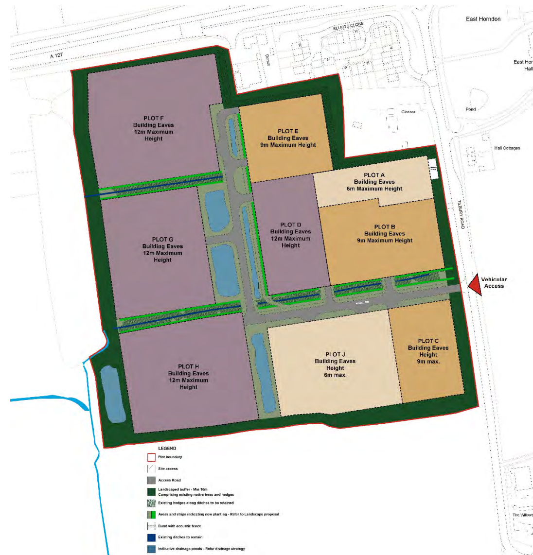
Plots and Landscape Parameters Plan – For indicative purposes only – Please refer to NWA-503-A03-010 drawing.
