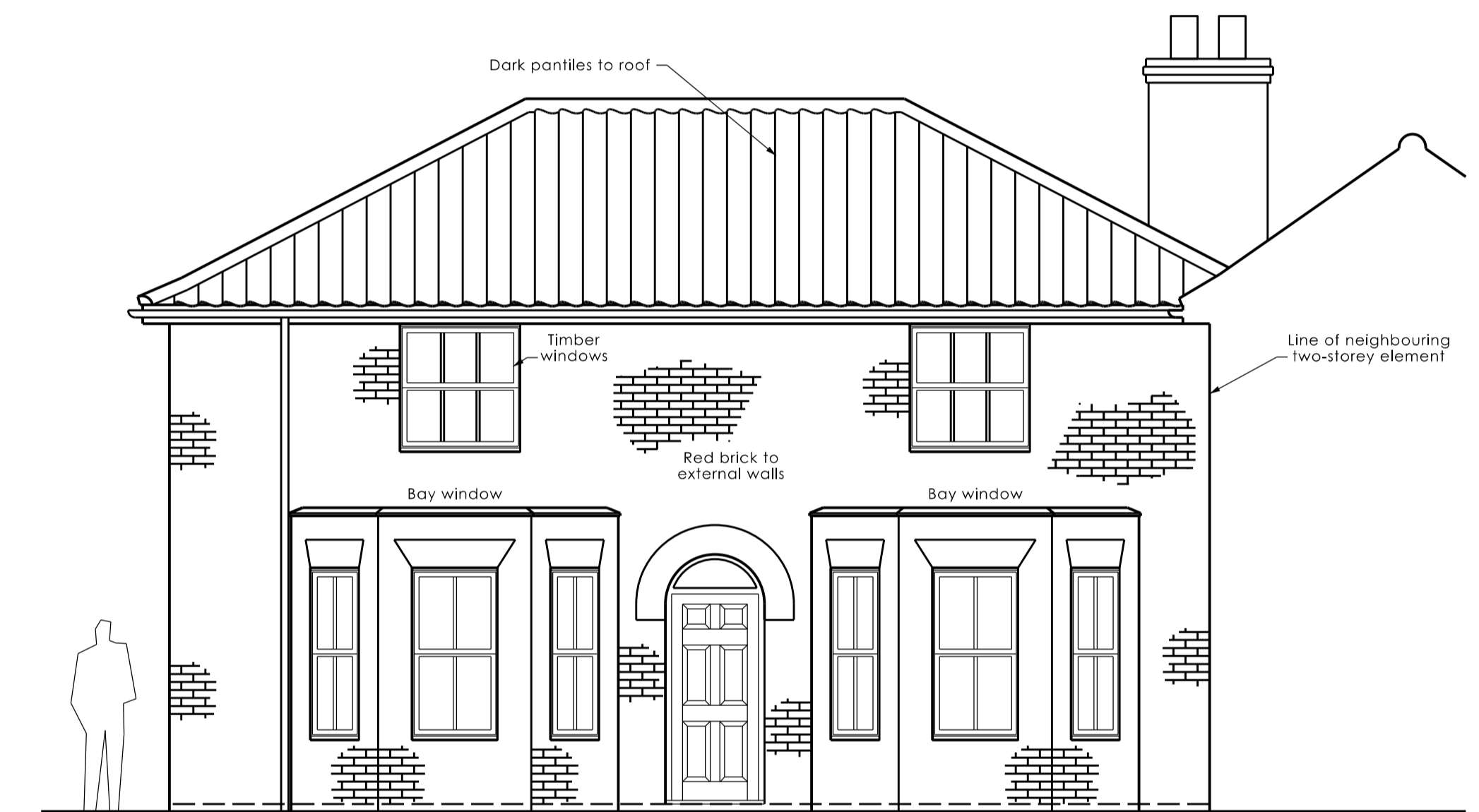
EXISTING EAST ELEVATION OF DWELLING 1:50 @ A1
