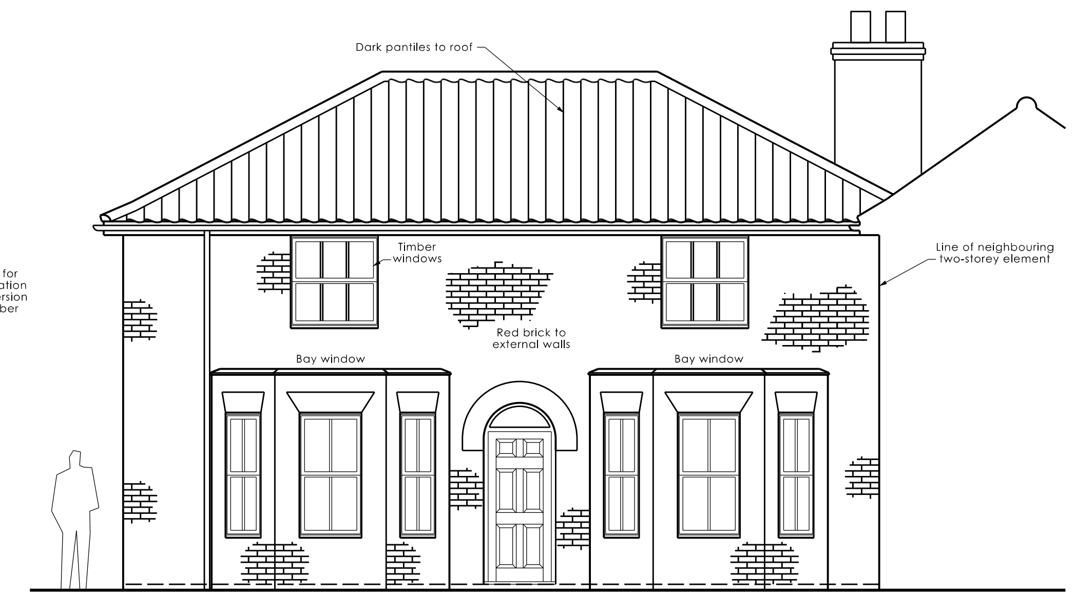
PROPOSED EAST ELEVATION OF DWELLING 1:50 @ A1 No amendments proposed to this elevation
