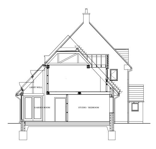
Roof Coverings Redland 'Stonewold' interlocking concrete tiles to match existing
