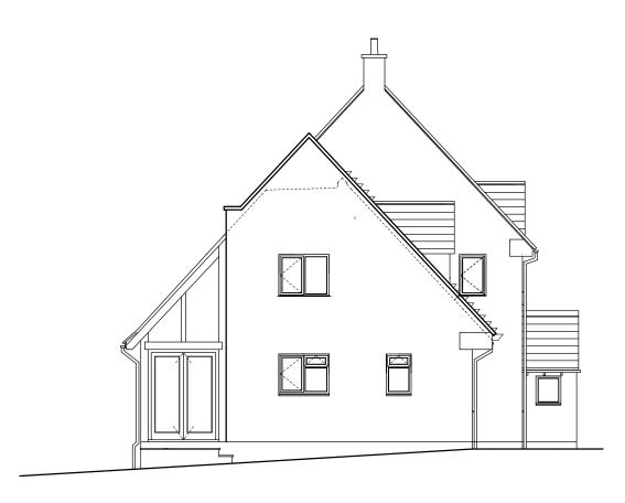
Roof Coverings Redland 'Stonewold' interlocking concrete tiles to match existing
