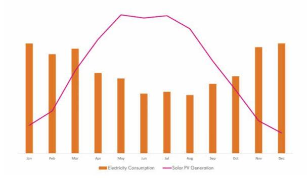
In the case of the North Rye House estate, summer loads for the pool building and future electric vehicle charging will result in more of the summer solar PV generation being used on site. If all purchased in electricity required to make up the shortfalls in the winter months is procured from a genuine zero carbon supplier, then the estate will potentially be carbon neutral for all energy demands, not just heat and potable hot water.
