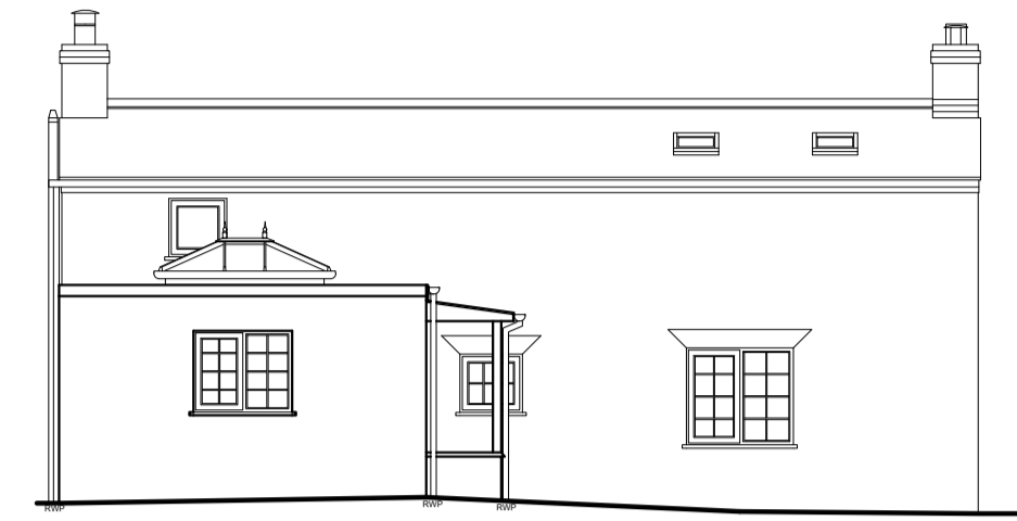
North Elevation - 1:100 0 1 2 3 4 5 6 7 8 9 10 Metres
