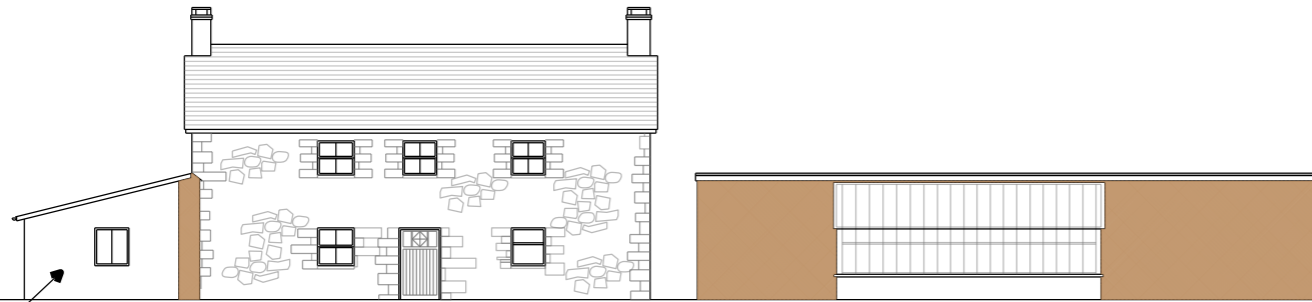
Extension is of shuttered concrete and or breezeblock construction.
