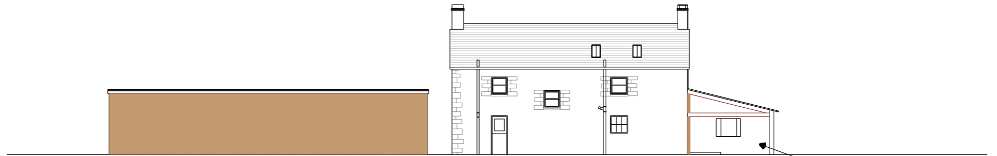
Elevation illustrating removed section of lean to building. Illustrated as a sectional elevation.
