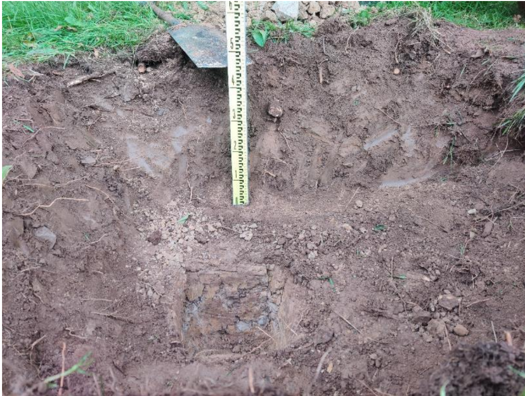
Fig 1. Trail hole 1, ruler showing invert of 500mm, 300mm hole just in front of this.
