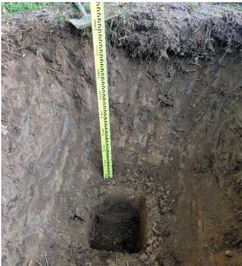
Fig 2. Trail hole 2, ruler showing invert of 800mm, 300mm hole just in front of this.
