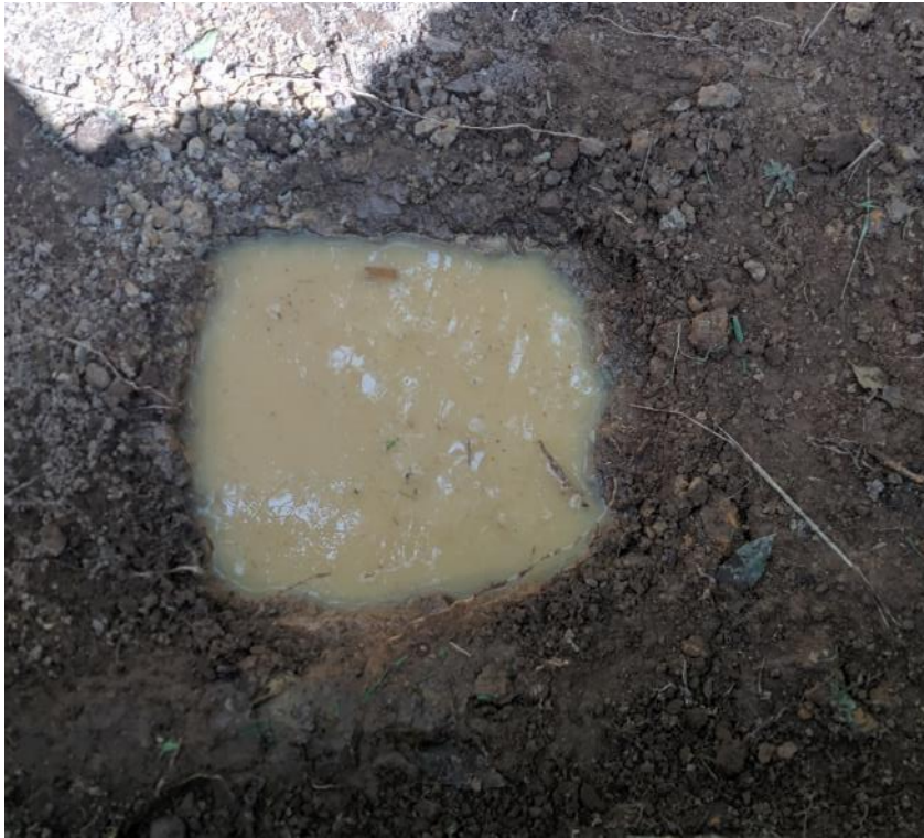
Fig 9. Trial hole 1 filled with water to just over 300mm
