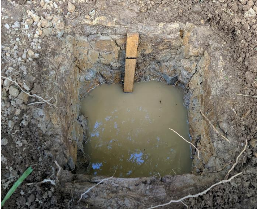
Fig 11. Trial hole 1 water reached first marker (25%), stop watch stopped.
