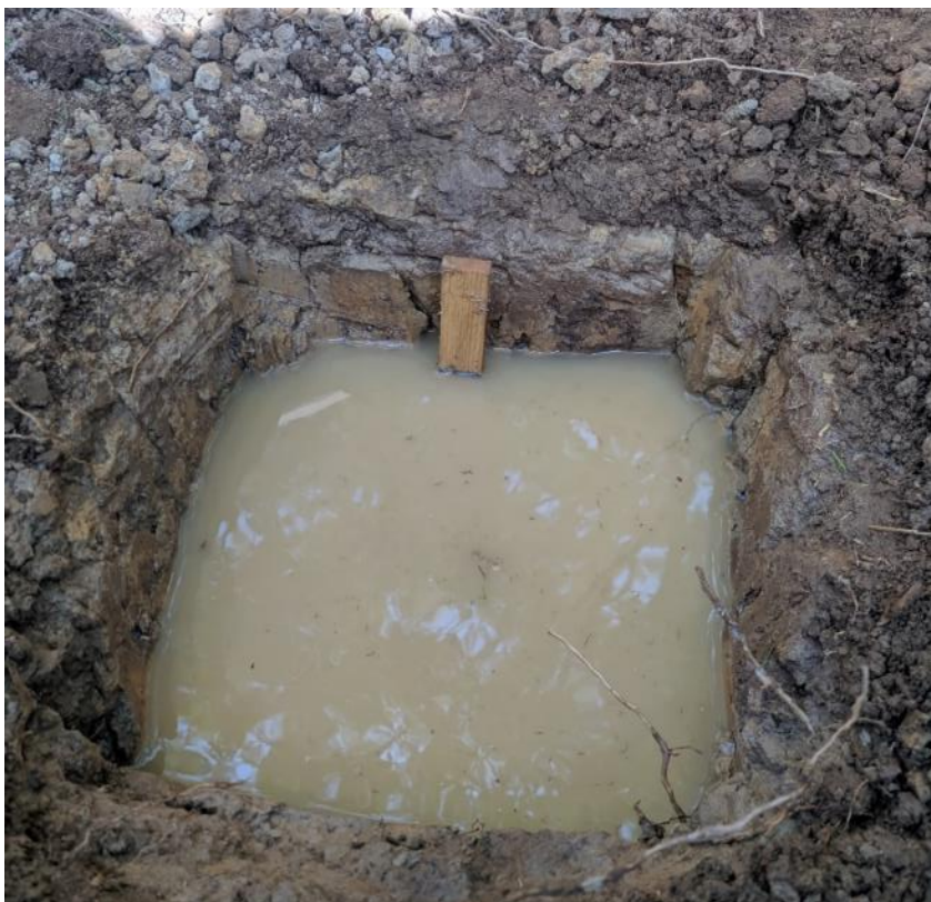
Fig 10. Trial hole 1 water reached first marker (75%), stop watch started.
