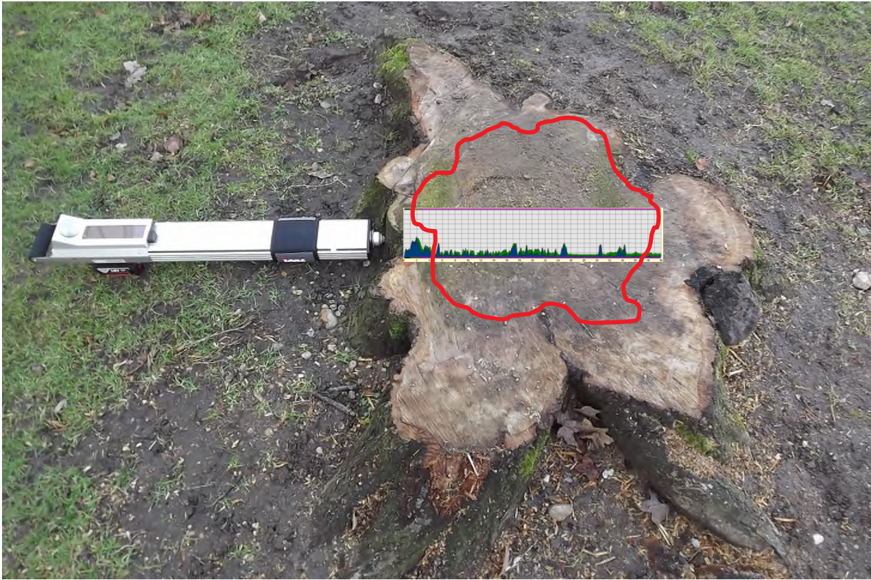
Resi Microdrill test of Lime tree stump
