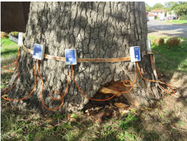
Open cavity with fungal fruiting bodies on south side of lower stem – Red line indicates scan level
