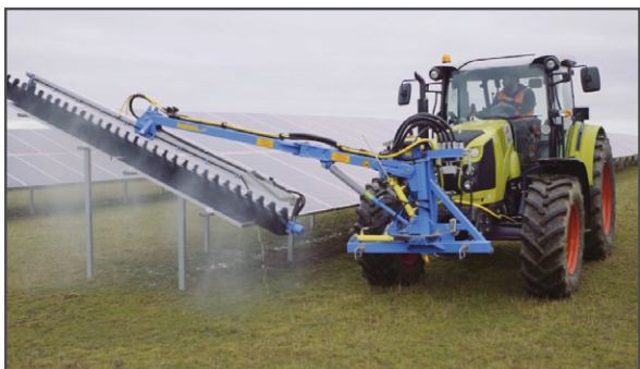
Plate 18 - Typical Solar Farm Cleaning Unit
