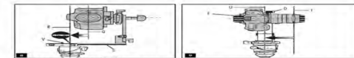
ADJUSTING PANORAMIC POSITIONING OF THE "METAL POINT" The "Metal Point" is the point where the panoramic axis of rotation intersects the vertical axis of rotation. It is the point where the camera's lens is positioned. To ensure accurate leveling of the head, the "Metal Point" must be perfectly aligned with the vertical axis of rotation. This is achieved by adjusting the knob "B" and the knob "Y".
