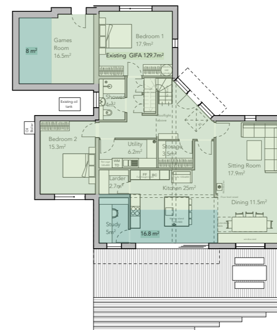
Proposed GF extension GIFA 24.8 m 2 Proposed GF total GIFA 154.5 m 2 Total GF GIFA increase 18%
