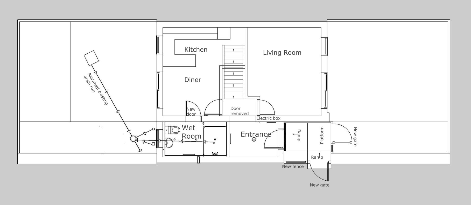
REF: PHELPS28062022 DFG ADDRESSS: 32 Crooked End Place, GL17 9YN CLIENT: Mr M. Phelps Proposed Ground Floor Plan REVISED 2 SCALE 1:50
