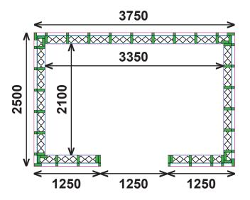
Floor Plan View Drawing No. 08 Scale 1:50 on A4
