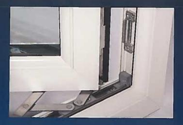
The addition of this simple device provides additional security on the weakest part of the window, the hinge. Their action of locking behind each other when the window is closed helps the hinges resist forced entry. By adding these and additional security features to Matrix 70 allows it to meet the requirements of Secured by Design.
