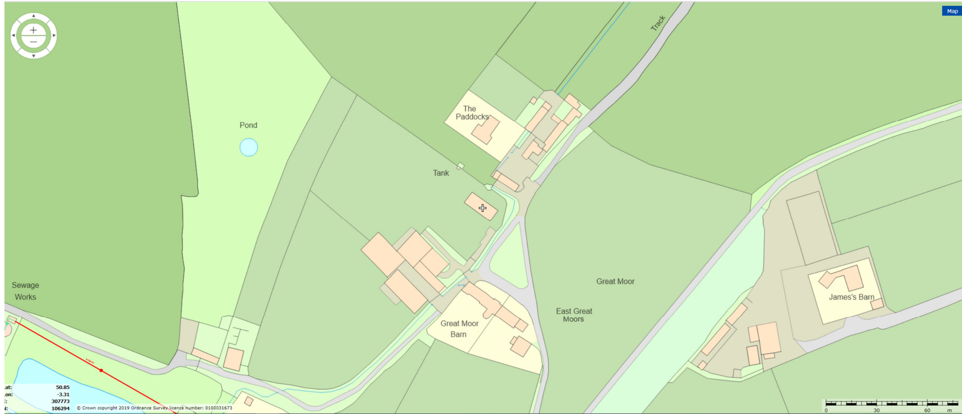
SWW Map extract – Confirming no mains sewer connection within 30m of the site.
