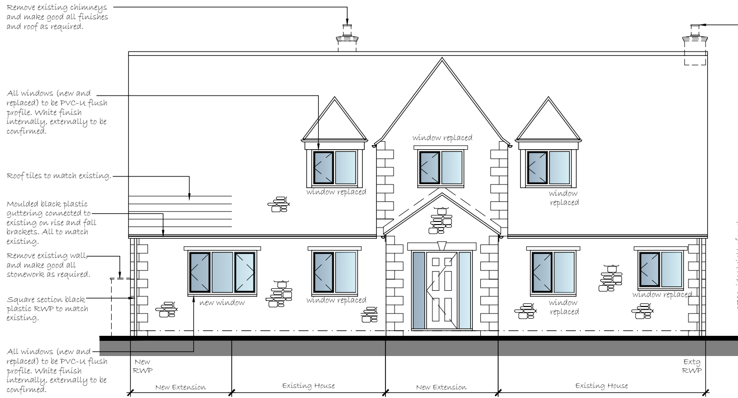
Front Elevation (west) @ 1:100
