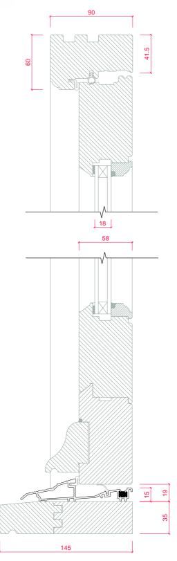
18mm Double Glazed Door - Open In Feature Mould: Ovolo Vertical Section Standard Threshold with 145mm x 35mm Projecting Cill
