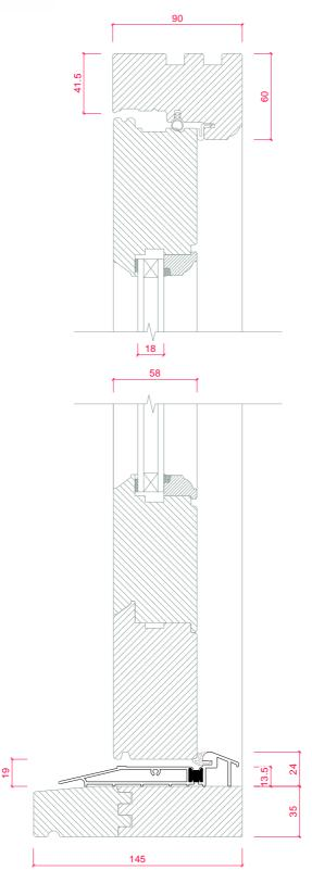
18mm Glazed Door - Open Out Feature Mould: Ovolo Vertical Section Standard Threshold with 145mm x 35mm Projecting Cill Style: IN-A-Stratfield Item Referen
