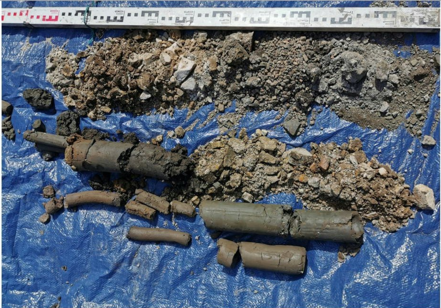
Image 1. WS03 runs : Viewed left to right and top to bottom: 0.00-1.00m bgl 1.00-2.00m bgl 2.00-3.00m bgl 3.00-4.00m bgl 4.00-5.00m bgl
