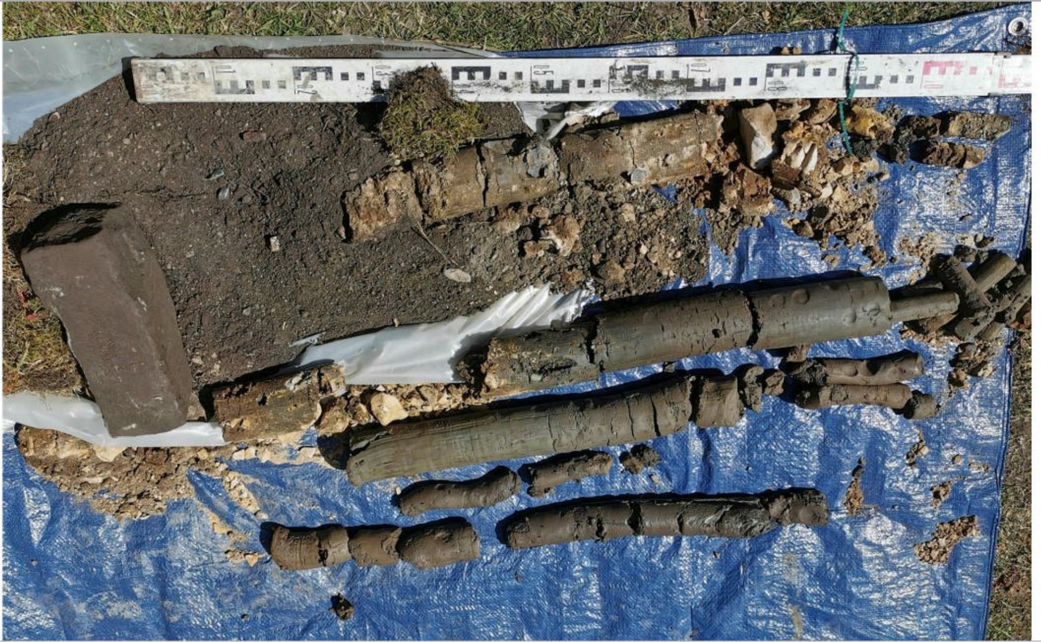
Image 1. WS02 runs: Viewed left to right and top to bottom: 0.00-1.00m bgl 1.00-2.00m bgl 2.00-3.00m bgl 3.00-4.00m bgl 4.00-5.00m bgl
