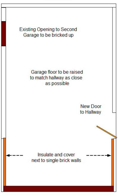
Existing garage door to be replaced with brick wall and window
