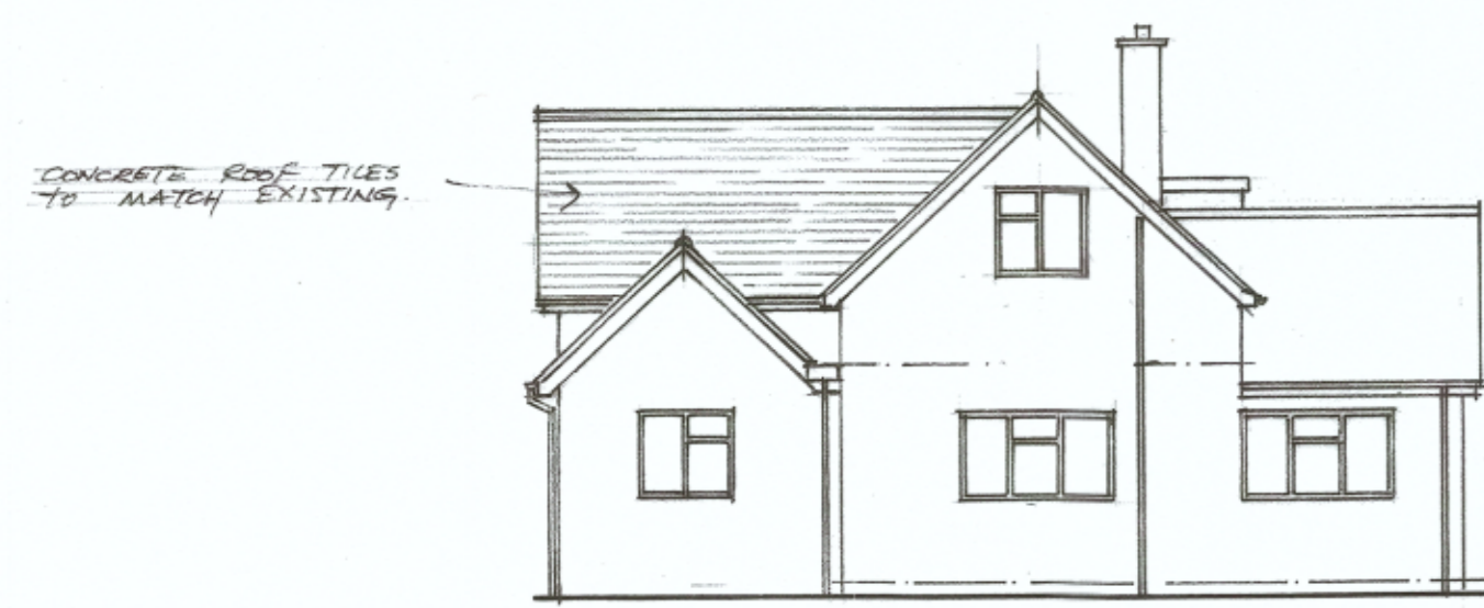
END ELEVATION (TO ROAD)
