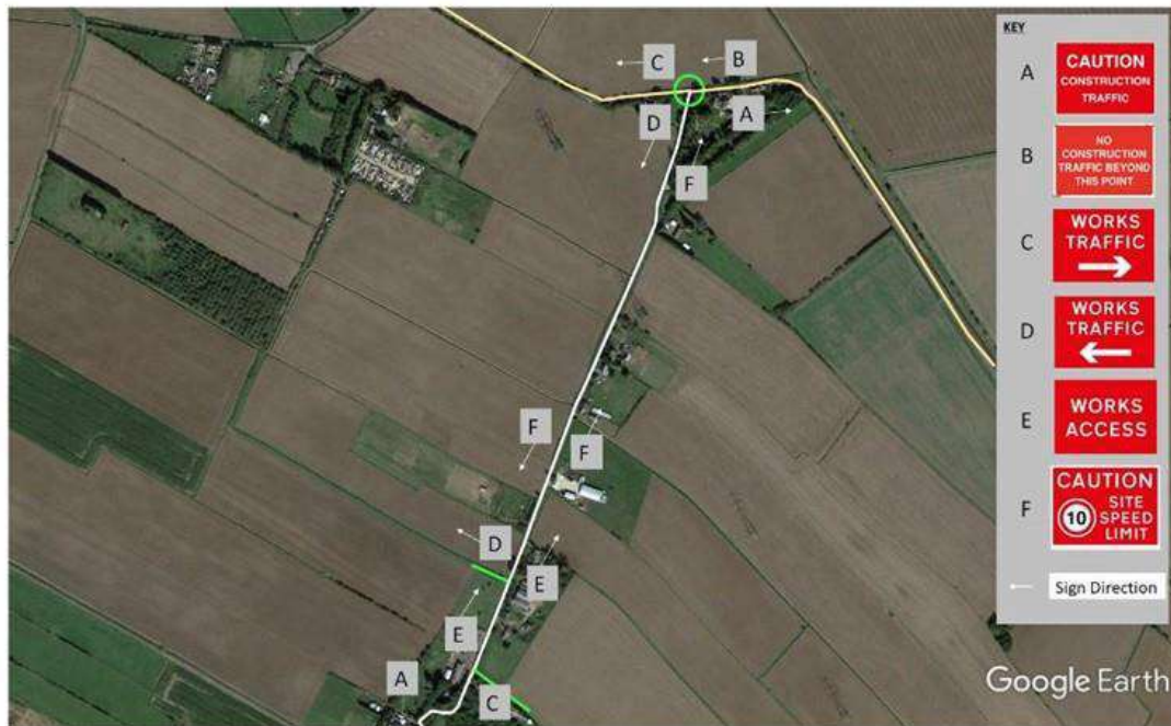
Figure 19. Harp’s Hall Road - Proposed Signage
