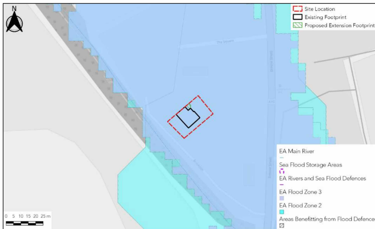
Figure 4: Site Specific Flood Zones from EA Flood Zone for Mapping GIS Layers (Source: OpenStreetMaps © Contains public sector information licensed under the Open Government License v3.0)
