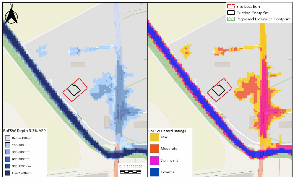
Figure 8: EA Surface Water Flood Risk Mapping 3.3% AEP (Source: Base map and data from OpenStreetMap and OpenStreetMap Foundation (CC-BY-SA). © https://www.openstreetmap.org and contributors, © EA copyright and/or database right 2015)
