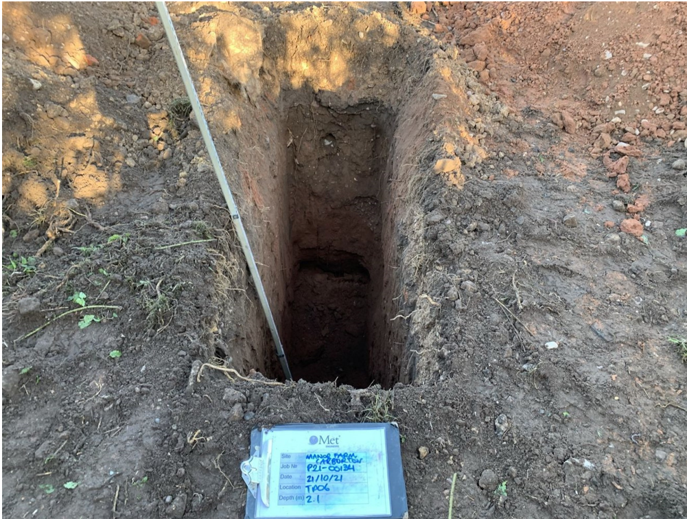
Photograph 17: TP06. Trial Pit.
