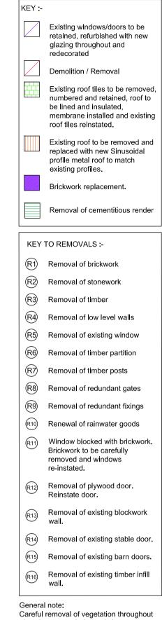
Careful removal of vegetation throughout elevations and missing pointing to be replaced with an appropriate lime based mortar.
