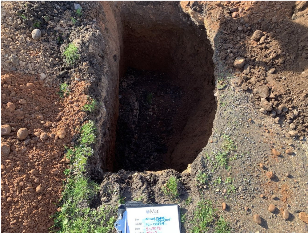
Photograph 08: TP03. Trial Pit.
