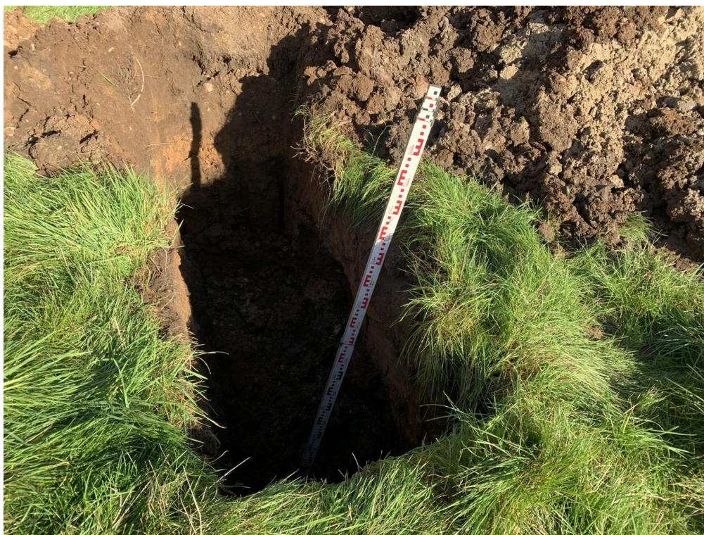
Photograph 39: TP13. Trial Pit.
