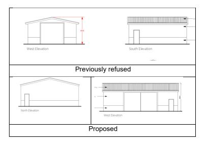
Stables. There would be no change to the stable size from the previous application. There would be three stables plus a tack room. The size would be 4.15m x 14.25m with a ridge height of 4.5m. Materials would be timber with a tiled roof.
