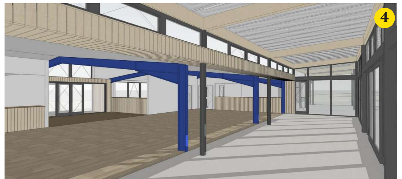
The rhythm of the existing portal frame continues into the new structure of the extension
