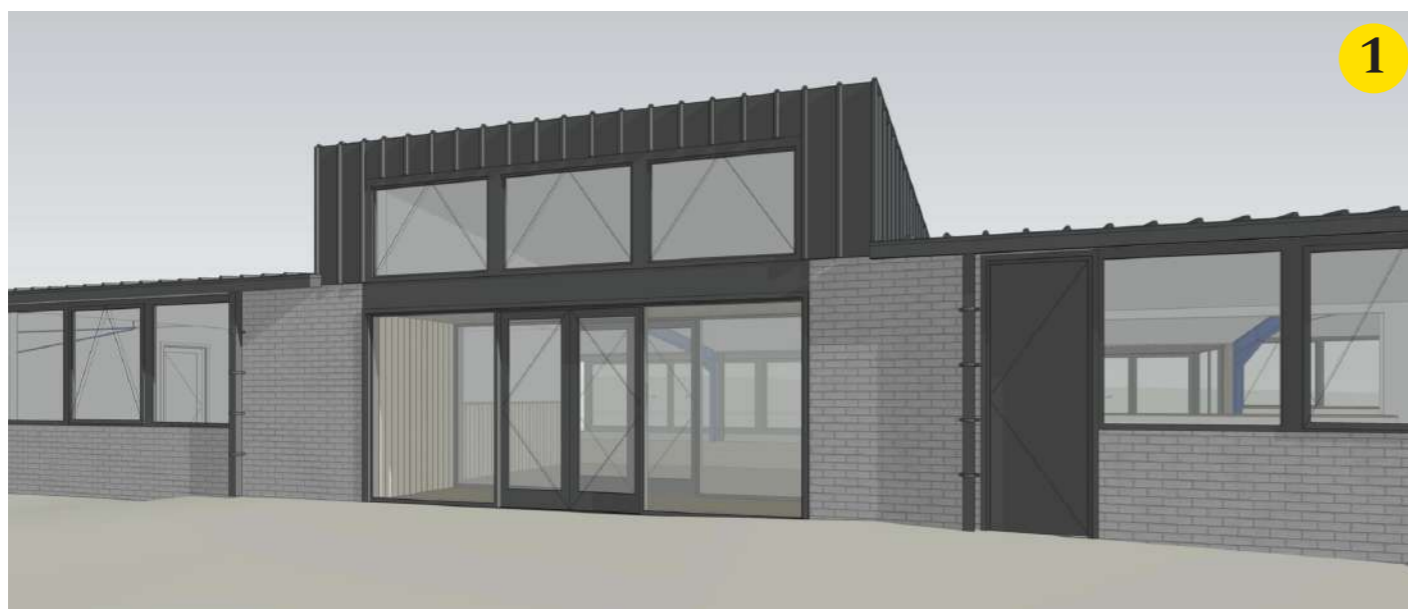
A dormer defines the new main entrance on the north elevation
