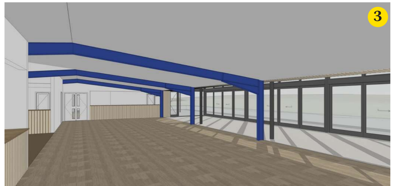
The interior layout is organised and defined by the exposed, rhythmic portal frame
