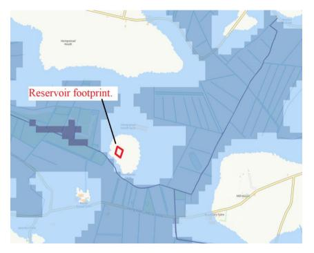
An uncontrolled release of water could only release 14,000 m<sup>3</sup> of water, this would run south into the Commissioners Drain. As can be seen the site has been chosen for its elevation above ground water and flooding.
