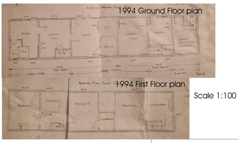
Proposal to remove recent stud partitioning on first floor. Partitions were added with planning permission in 1994/5. Returning the property to its original layout with the reinstatement of an oak staircase and ground floor WC, again as was insitu prior to 1994.
