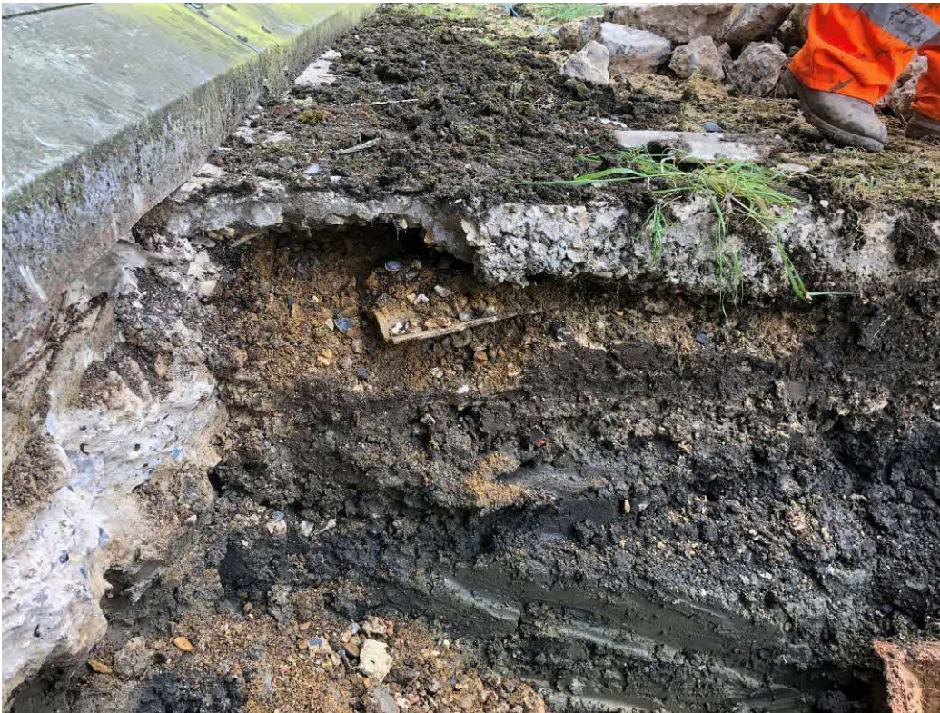
Photograph 4 – Fragments of asbestos cement taken from the side of TP203
