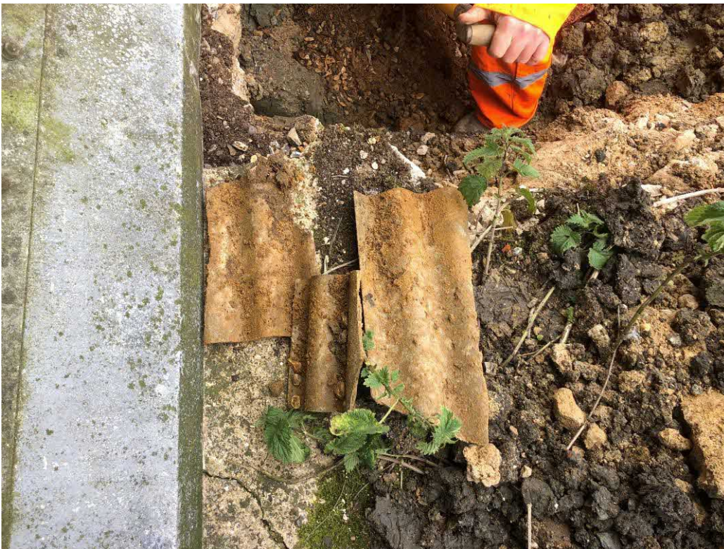
Photograph 4 – Fragments of asbestos cement taken from the side of TP203
