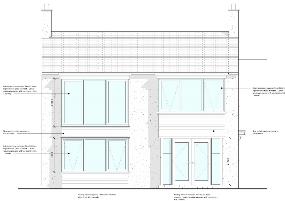
Proposed elevation detailing alterations to existing windows
