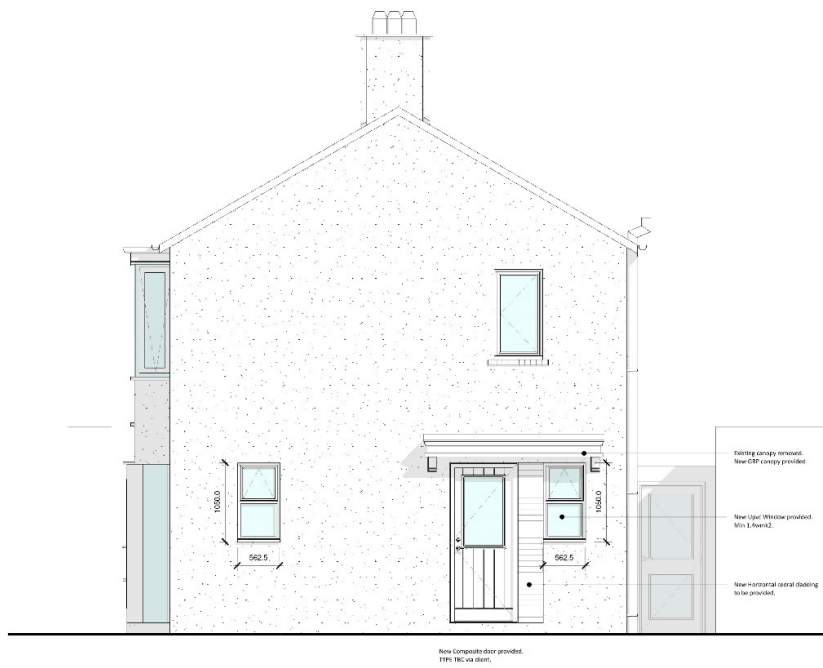
Proposed elevation showing new alterations including alteration to rear door and installation of new Canopy.
