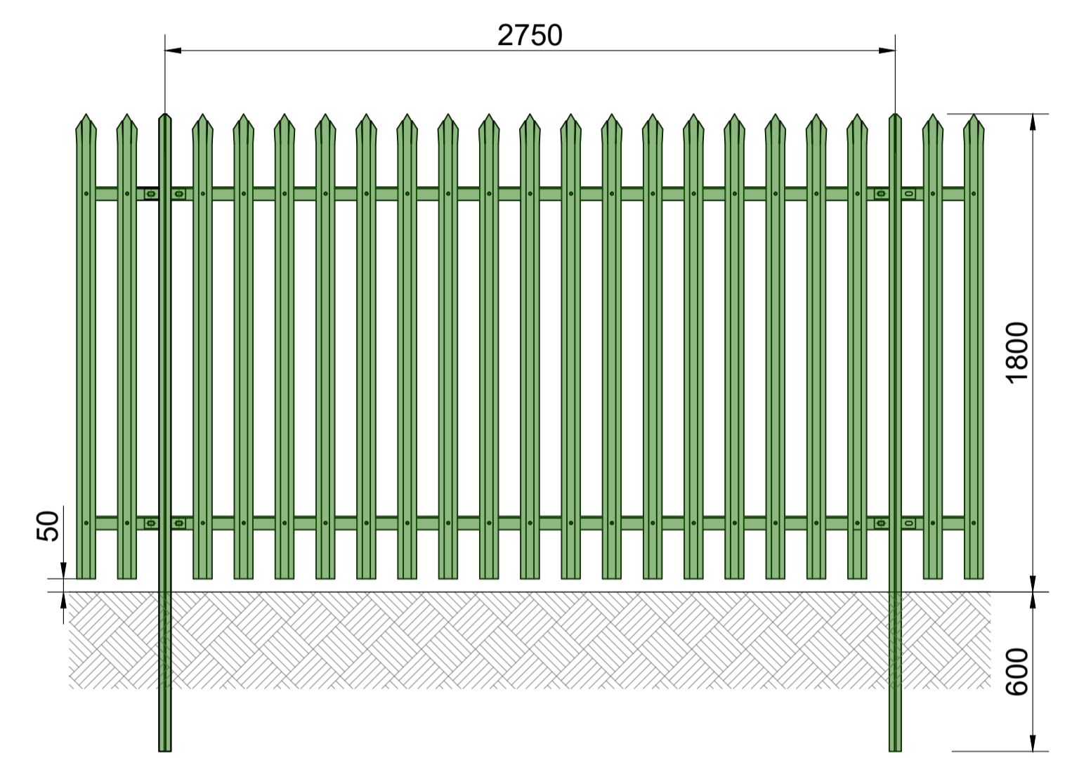
Palisade Fence Elevation 1:20 New Fence finished in RAL 6025 'Fern Green'
