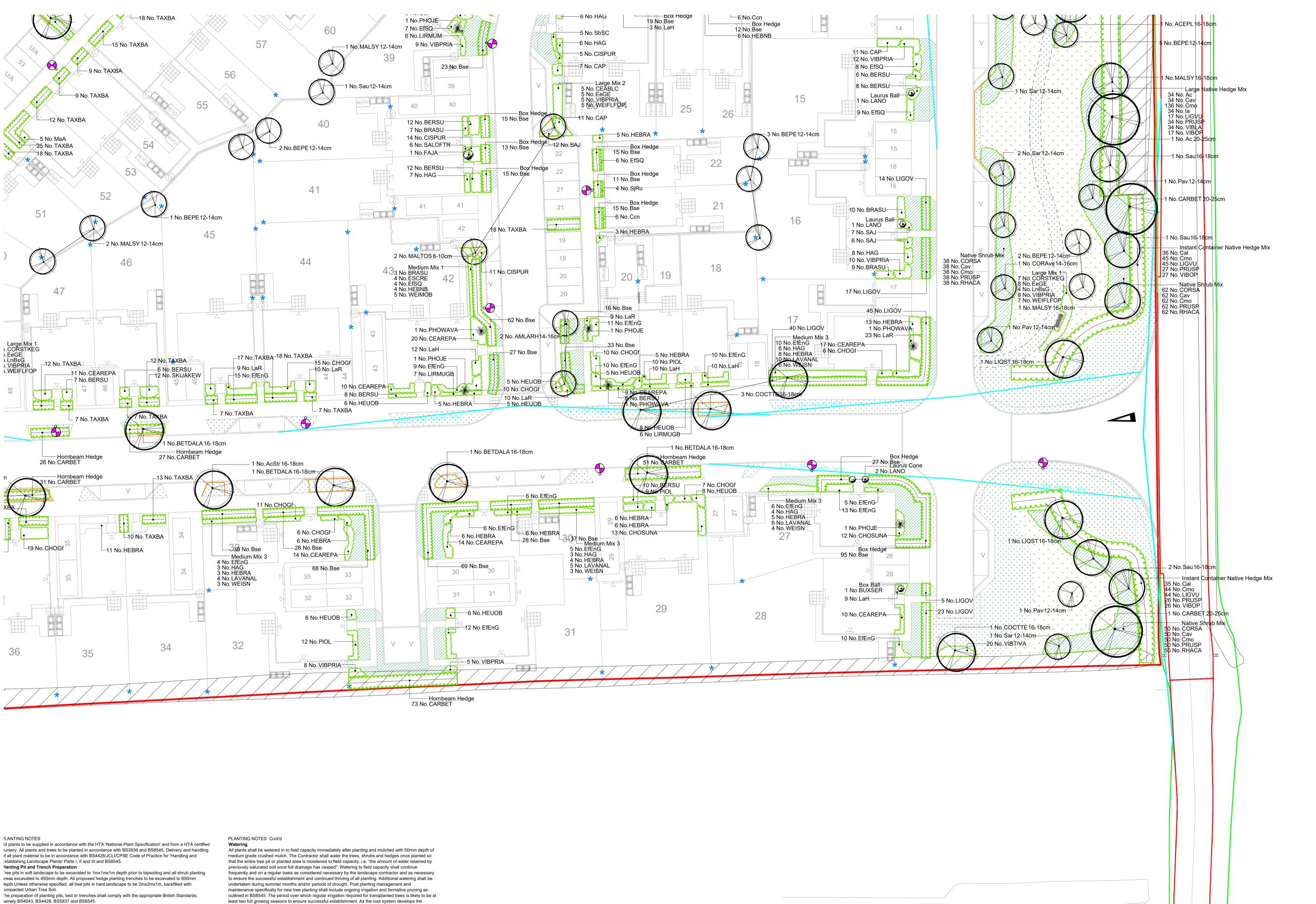
reas excavated to 450mm depth. All proposed hedge planting trenches to be excavated to 600mm lepth.Unless otherwise specified, all tree pits in hard landscape to be 2mx2mx1m, backfilled with
