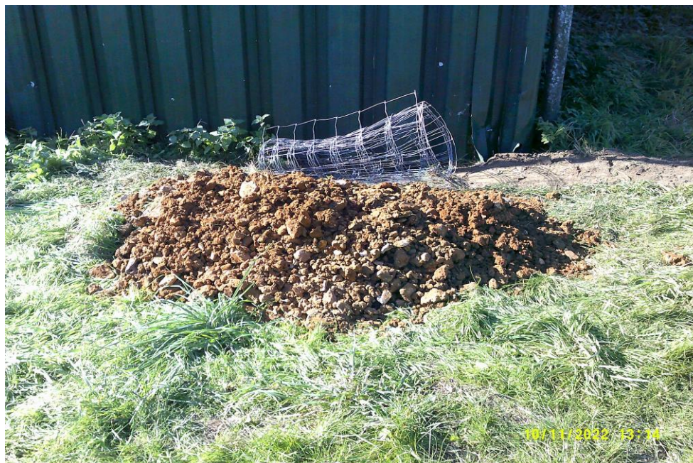
Frame No: 05 Location: The Cold Store, Butlers Farm, Horseshoes Lane, Maidstone, Kent ME17 3JY Description: The material from the trial pit in photo 4, a stone clay head material Date: 11/10/22
