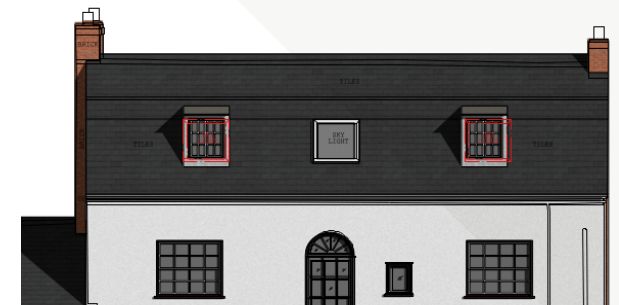
REAR OF PROPERTY - New dormers will be introduced to match those at the front of the property.
