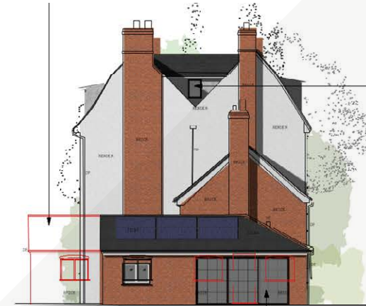
SOUTH ELEVATION (Side) - The south shows the partial removal of the existing garage as well as a new set of Crittall glazed doors.
