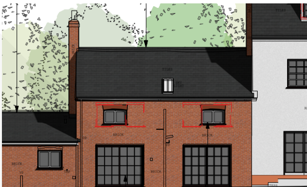
REAR OF PROPERTY - New Timber windows will be more sympathetic in scale, matching the windows to the front of the property.
