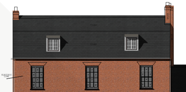
FRONT OF PROPERTY - two new dormer windows reinstate the positions of historic dormers - see Fig 9. From Historic Asset Assessment (above).
