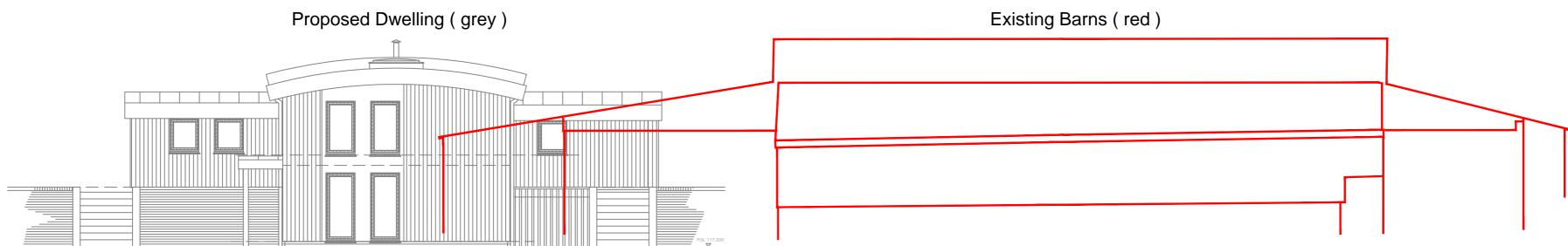
North Elevation of Proposed Dwelling (grey) Showing Existing Barns (red) Scale 1-100 THE CONTRACTOR IS RESPONSIBLE FOR CHECKING ALL DIMENSIONS ON SITE ANI IS TO REPORT ANY DISCREPANCY TO THE CONSULTANT PRIOR TO THE COMMENCEMENT OF ANY WORKS.
